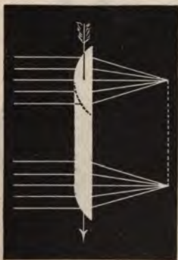
FIG. 162.—The Action of a Convex Cylindrical Lens upon Parallel Rays.
